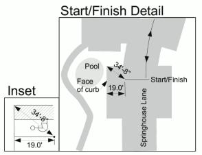
Start and Finish is 19'-0" from face of granite curb along the first ADA parking space as shown; also 34'-8" from corner of granite curb. Parking space is along Springhouse Lane, just east of the bike rental desk and pool.
